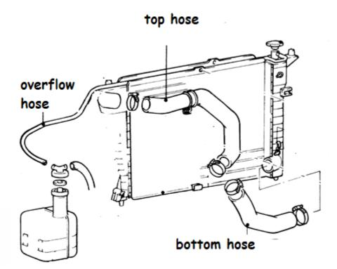
Hose clamps are used to secure the hoses to their outlet or inlet fittings. Additional hoses to the heater will also be fitted. **Frost** or **Welsh** plugs are fitted into the block and cylinder head after their manufacture to fill the casting holes from manufacture. These plugs are often into coolant jackets so they are sealing the coolant into the jackets.
