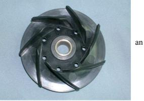
The coolant pump can be driven by a system of pulleys and belts taking the drive from the crankshaft of the engine, or electrically by an electric motor.
