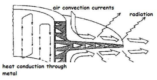
Conduction occurs as the piston and burning air / fuel in the cylinder produce heat in the cylinder. This heat is conducted through the cylinder fin.
