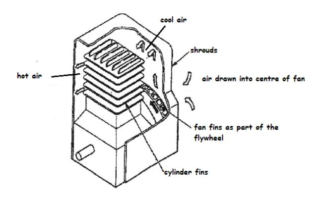
Although no longer in production because of the inefficiencies of air cooled systems, manufacturers like Porsche and Volkswagen used direct cooled for many years with larger displacement engines and high performance engines. These larger displacement engines often had additional flaps that operated in the cooling shrouds to open and close to help control the engine temperatures.
