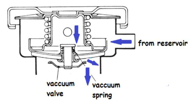
A major benefit in regard to this system is that air is eliminated from the cooling system, any air in the system would alter the temperatures and pressures.
