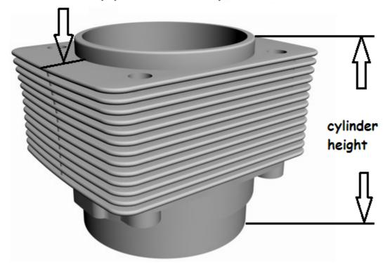
See how the overall distance is around the fins is far greater than the distance of the cylinder height and the surface area of the fins is huge compared to the surface area of the cylinder.
