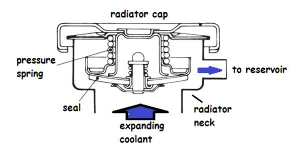
As coolant escapes the radiator past the cap seal it is collected in the reservoir bottle or header tank as it is sometimes called.
