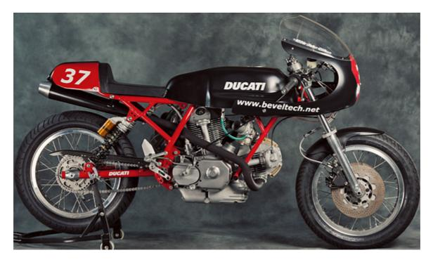
Imagine this Ducati moving through the air, the fins on the cylinders, cylinder heads and sump fins are lined up to allow the air to flow over them but it the bike stops moving and is still running then air flow becomes nothing.
