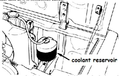
The pressure spring in the radiator cap is able to maintain the coolant system pressure at the specified level, **but now what happens** when the engine is switched off and cools down?
