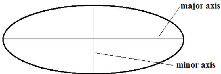
Because the diameter and radius don't work for an ellipse, we say it has a major axis (the distance across the widest part lengthways) and a minor axis (distance across the widest part crossways)
