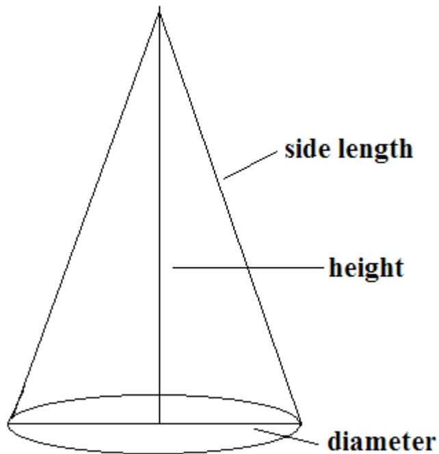
A **cone** has a shape like an ice-cream cone. It has a diameter across the open end, a height from the centre of the diameter up through the tip of the cone, and a side length which is from the outer edge to the tip.
